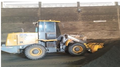
Gambar 5. Metode kerja Wheel loader ( V-Cut )
