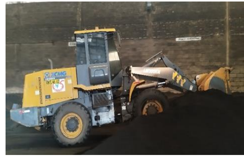
Gambar 6. Metode kerja Wheel loader ( Dozing )
