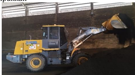
Gambar 1. Metode wheel loader ( Load and Dump )
