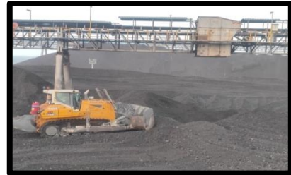
Gambar 9 Dozing material masuk lubang vibrating
