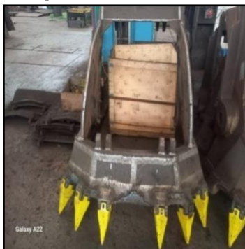
Gambar 10. Finishing pebaikan bucket
