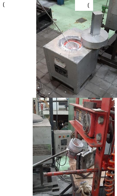
Gambar 4 (a) Proses peleburan (b) Proses squeeze casting
